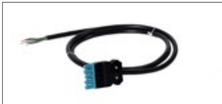
Mains cable, Wieland, 5-pin. 1-phase + dimming. L = 2.0 m with female, 5 x 1.5 mm 2 .
