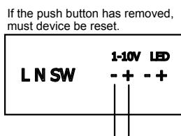
Short circuit 1-10v port for min 2 sec to reset the device
